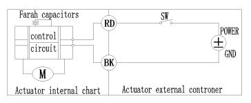
• When SW is closed , the valve open. the actuator automatically power off after in place
