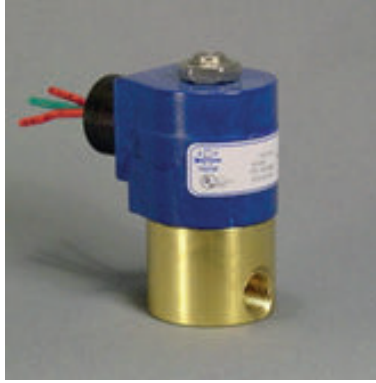
S30 & S31 Direct Acting 1/4", 3/8", 1/2" Brass or Stainless Steel 0 to 2400 psi Water 0 to 150 psi Steam
