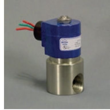
S40 Piloted Piston 1/8", 1/4", 3/8" Brass or Stainless Steel 0 to 300 psi Water 0 to 150 psi Steam
