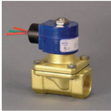
S21 Piloted Piston 3/8" to 2" Brass or 316 Stainless Steel 4 to 150 psi Water 4 to 50 psi Steam
