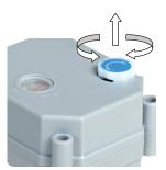
In case of an electric supply failure, it is possible to operate the actuator manually:
